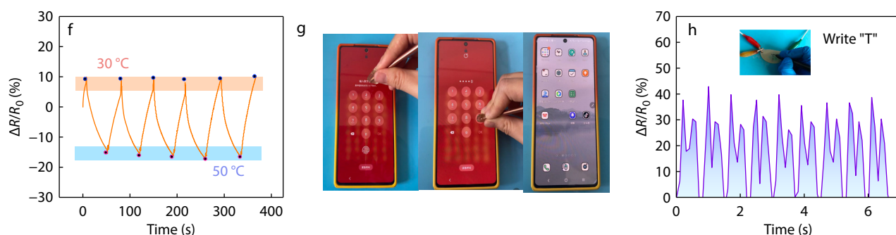
Fig. 6 (a) The relative resistance change curves and (b) GF of the gel based sensors at different strain ranges (100%–400%) and (c) stretching 100 cycles at 50% strain; (d) Underwater sensitivity and (e) temperature coefficient of resistance (TCR) of the PPAS-Al 3+ gel; (f) Resistance change curve under 10 cycles at 30 and 50 °C; (g) The gel sensors used as an electronic contact pen to simulate the phone unlocking process and (h) relative resistance change of the gel-based writing pad during handwriting of the letter "T".
